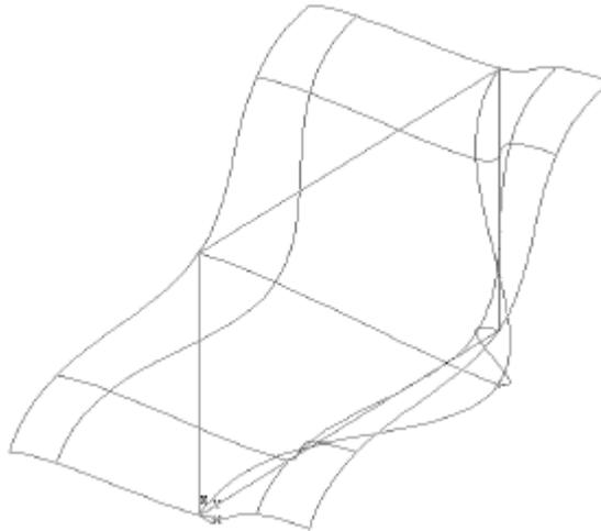
Figure 17. A surface generated from four curves and a point.
