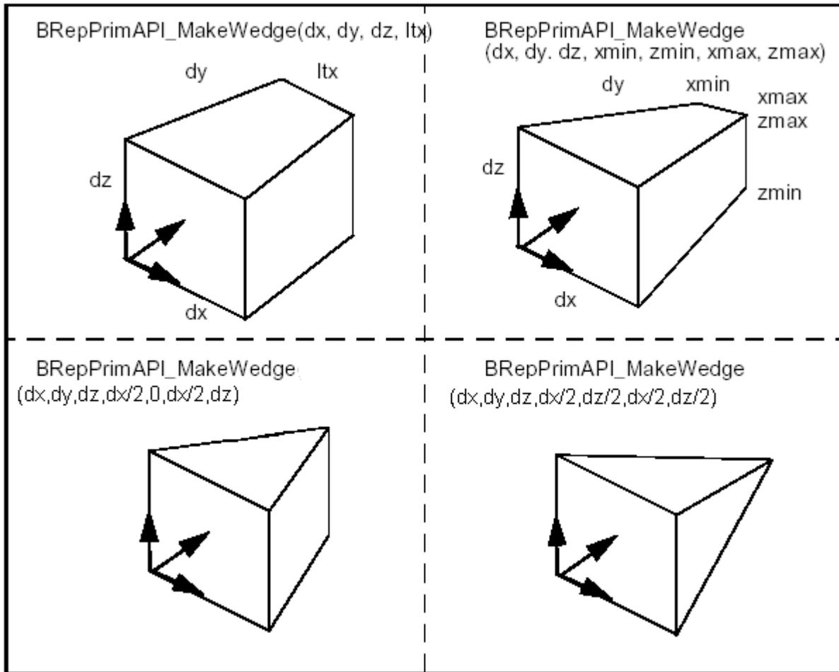
Figure 25. Making Wedges
