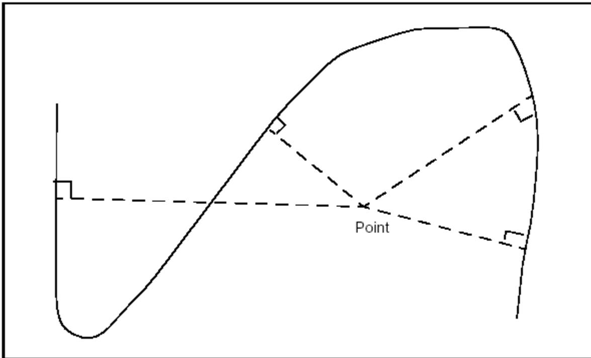
Figure 18. Normals from a point to a curve
