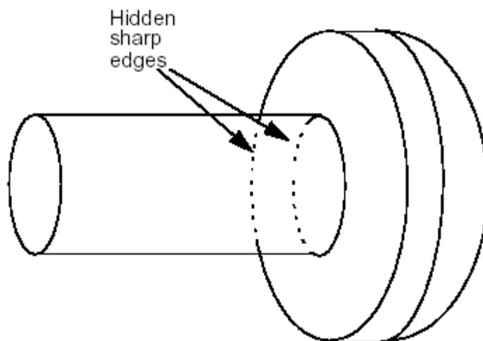
Figure 53. An extraction showing hidden sharp edges
