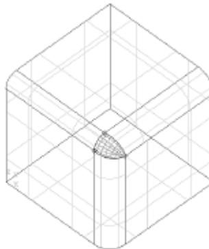
**Figure 16. Intersecting filleted edges with differing radii, presenting a gap which has been filled by a surface.**
